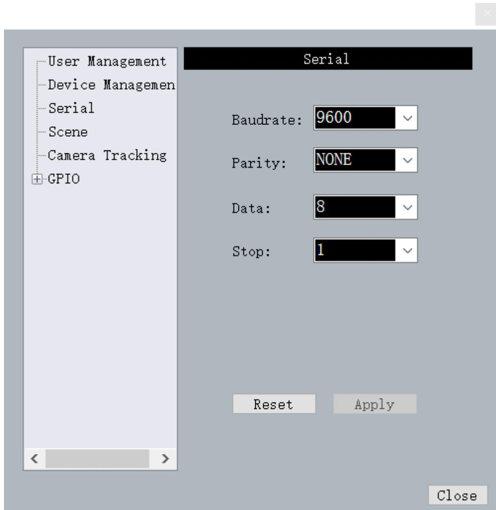
View and modify the serial port information of the current device. Click "Apply" button to modify the serial port information of the current device after setting; If you want to return to the default value, directly click the "All Reset" button, and the items cannot be empty when setting.
