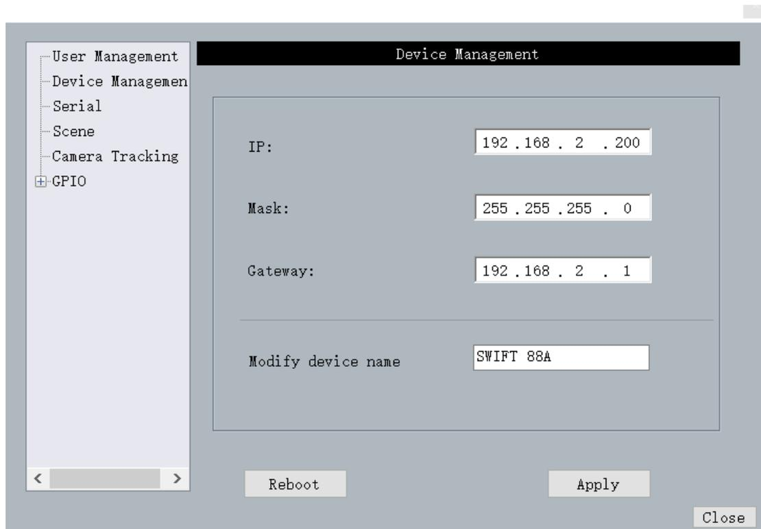
The screenshot shows a web-based interface for "Device Management". On the left is a navigation menu with the following items: "User Management", "Device Management", "Serial", "Scene", "Camera Tracking", and "GPIO" (which is expanded with a plus sign). The main content area is titled "Device Management" and contains the following fields:
